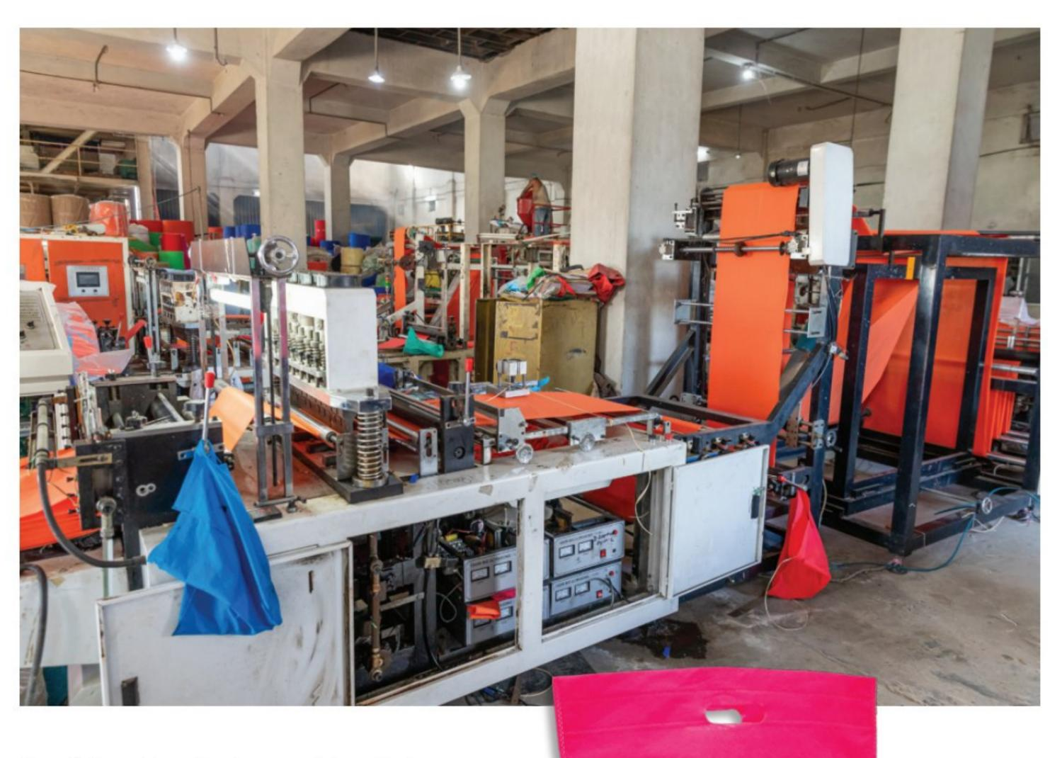
Our fully automatic bag machines help us manufacture non-woven shopping bags in various sizes as well as designs like U cut, D cut, loop handle, box type and many more with accuracy and high-quality. All the seams and handles are machine finished, making it durable and long lasting.
